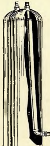
Shows how Aquatherm leads hot water direct from heater into service lines.
