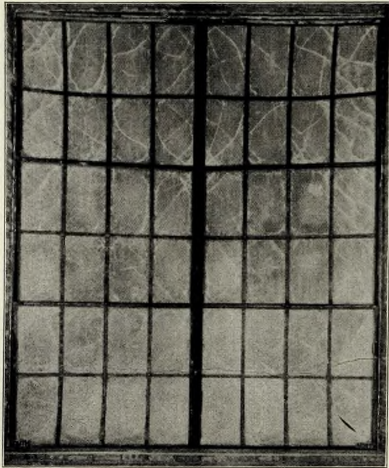
Large type of fire window with 2-in. mullion listed after a successful test.
