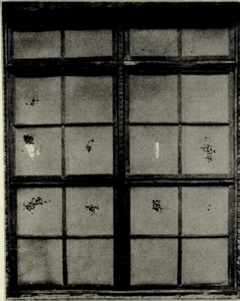
New type of fire window and transom having only a 2-in. mullion which tested out satisfactorily.
