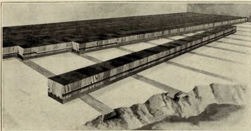
Perfect Installation Over Concrete with Imbedded Sleepers
